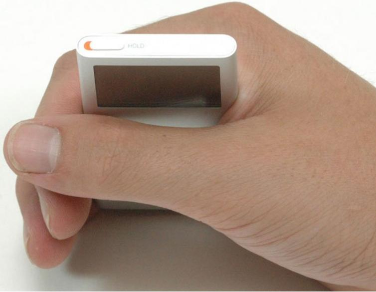
ⓘ Before opening your iPod, ensure that the hold switch is in the locked position.
