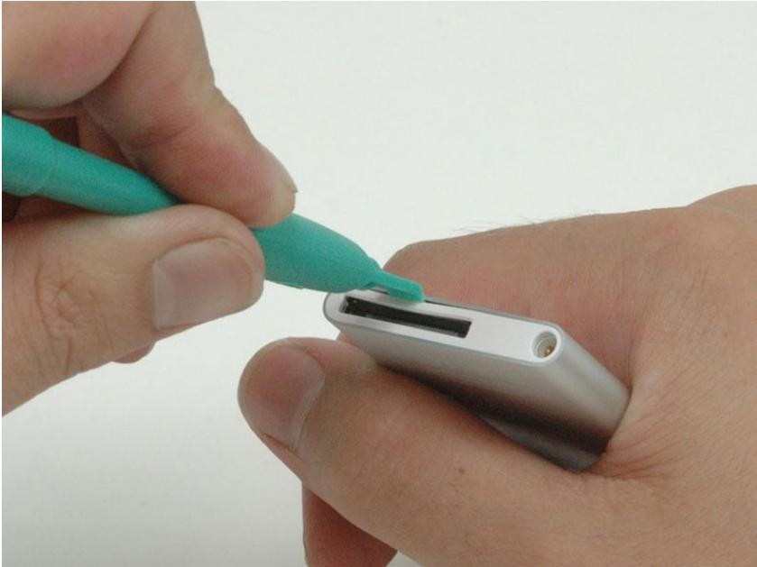
⚠ When removing the the bottom bezel, be sure not to bend the plastic surrounding the dock connector.
