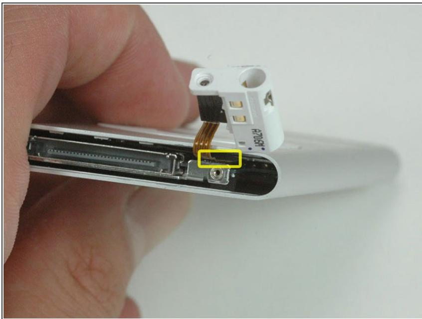
ⓘ The highlighted connector attaches the click wheel and headphone jack to the logic board. This cable must be disconnected from the logic board before continuing.
