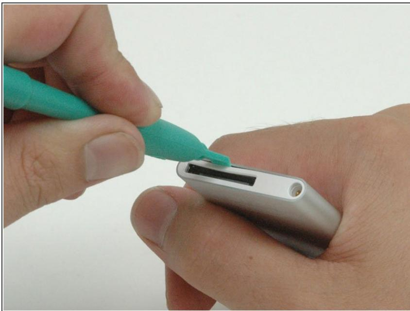
**⚠** When removing the bottom bezel, be sure not to bend the plastic surrounding the dock connector.
