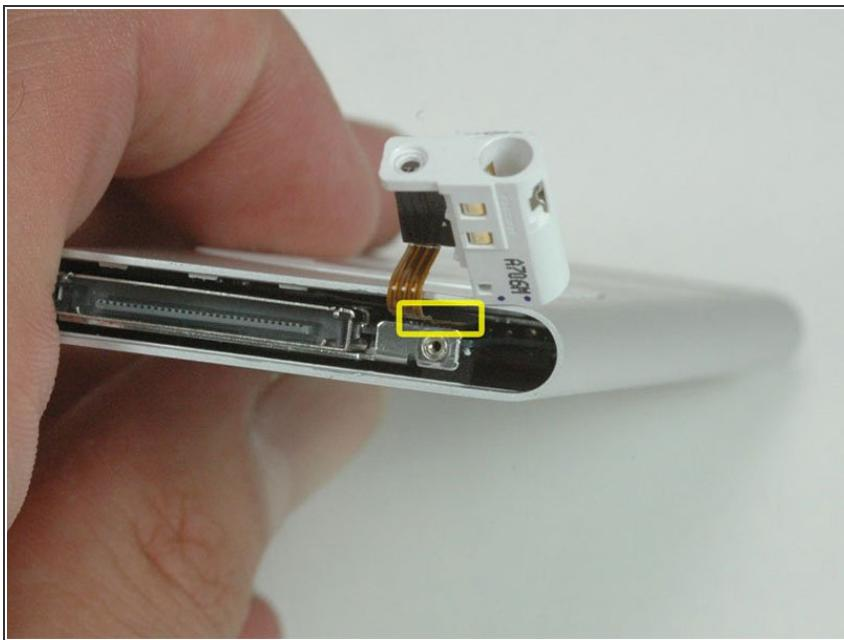
**i** The highlighted connector attaches the click wheel and headphone jack to the logic board. This cable must be disconnected from the logic board before continuing.
