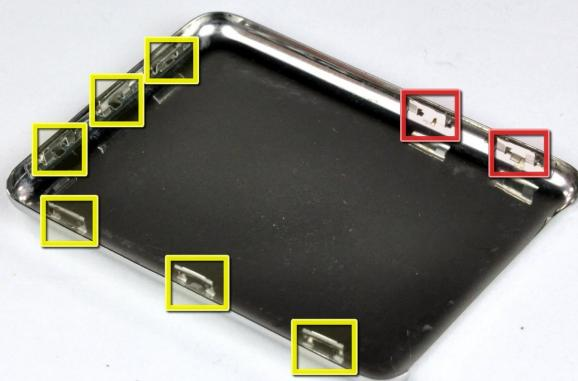
**i** The rear panel is secured to the front case by eight clips permanently attached to the rear
