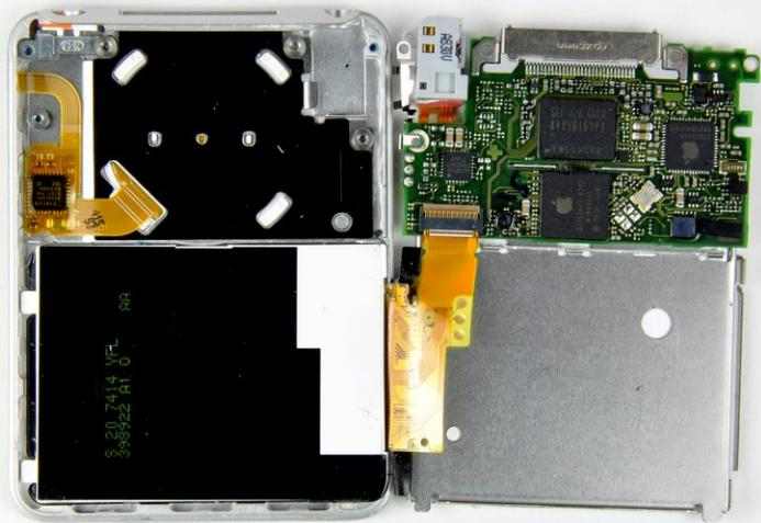
**⚠** The logic board is still connected to the front case by the display ribbon cable, located on the headphone jack side of the logic board.
