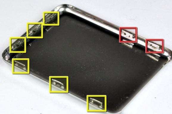
**ℹ** The rear panel is secured to the front case by eight clips permanently attached to the rear
