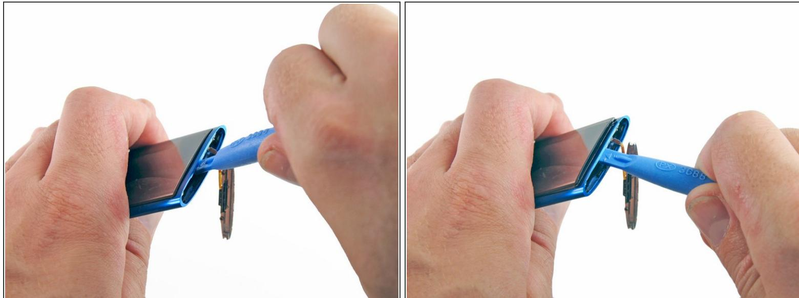
*(i)* The glass panel is held in place by adhesive on all four sides. In the following steps, work carefully to avoid cracking the glass.
