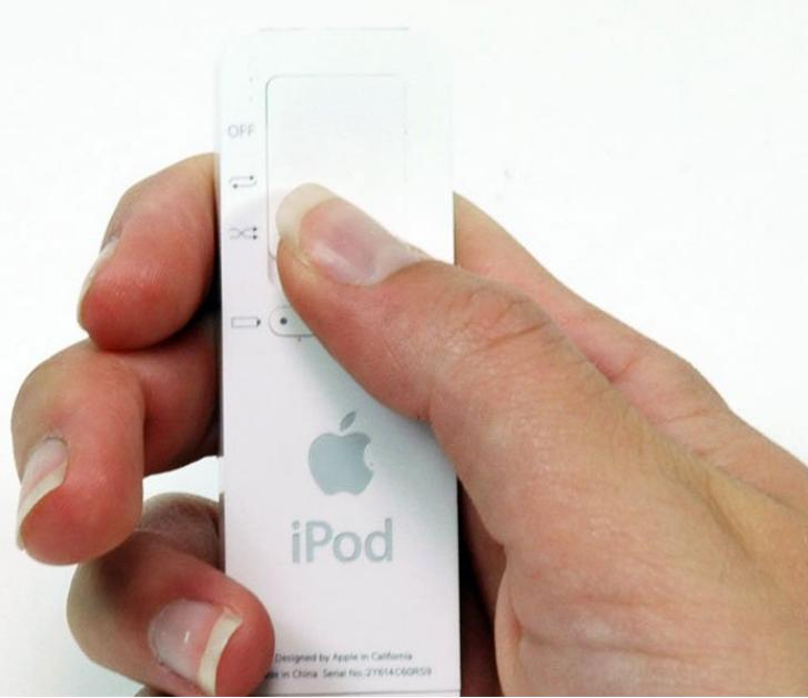
ⓘ Before opening your iPod, ensure that the hold switch is in the locked position.
