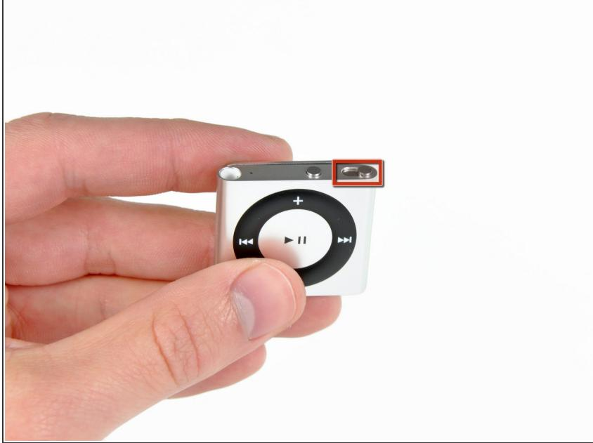
**⚠** Accessing the internals of the 4th generation Shuffle is extremely difficult, as the rear panel is both glued to the front case and secured by metal retaining clips. It is highly unlikely that you will be able to remove the rear panel without inflicting cosmetic and/or structural damage.
