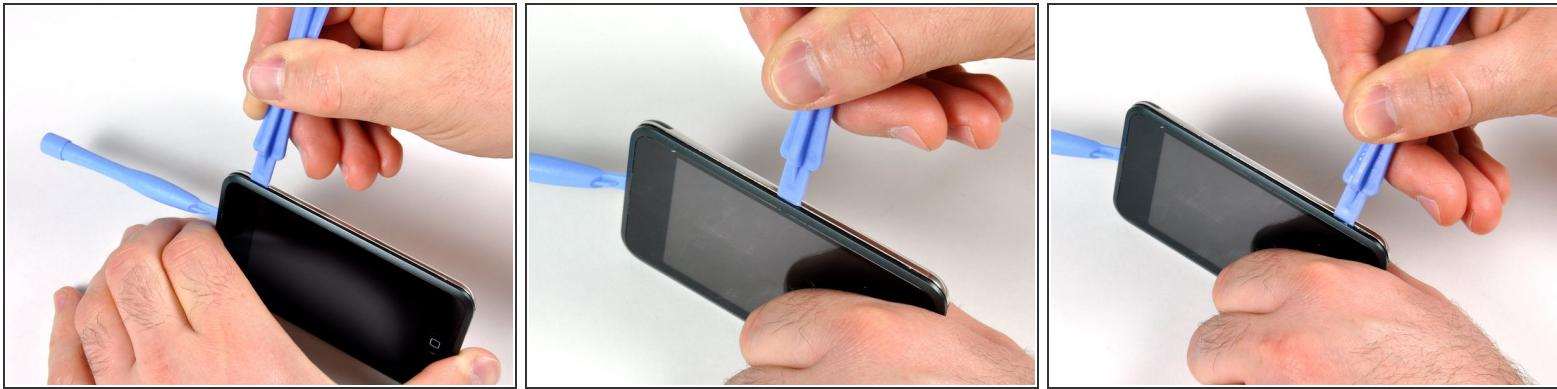
ⓘ There are seven interlocking retaining clips on each side of the iPod. The large plastic opening tool will be used to separate the front panel from the metal back of the iPod.
