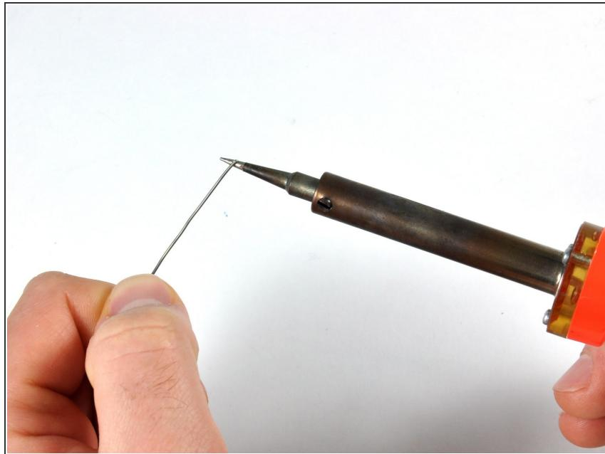
**i** We're now ready to begin the soldering process. You'll need a soldering iron, solder, and desoldering wick. You should be able to find these items at a Radio Shack if you don't already have them.
