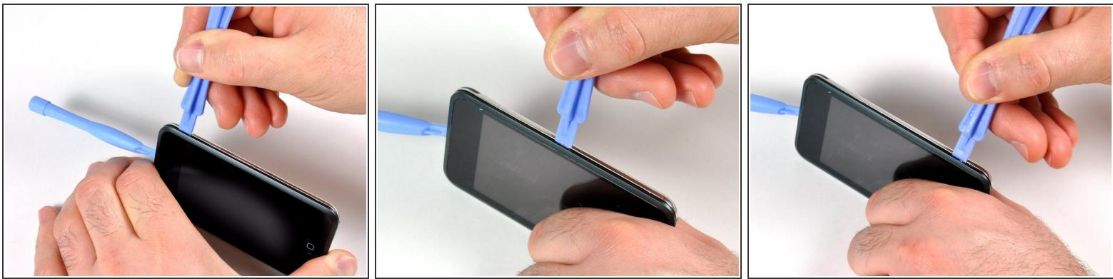
① There are seven interlocking retaining clips on each side of the iPod. The large plastic opening tool will be used to separate the front panel from the metal back of the iPod.
