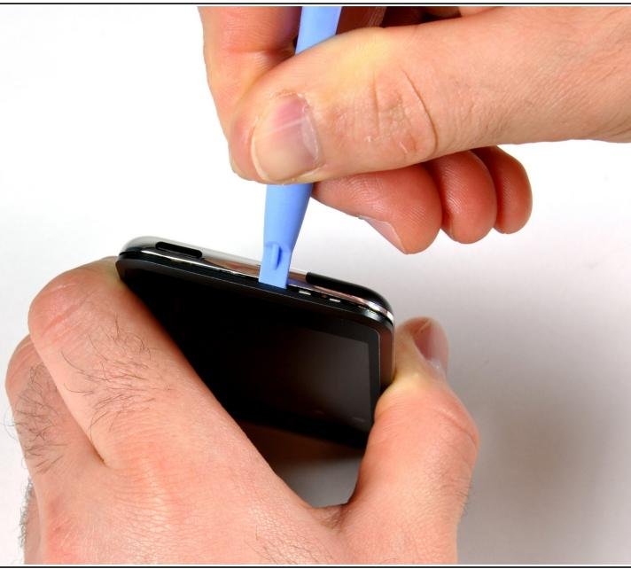
! Opening the case is a tough and potentially dangerous task. A good amount of force is required to wedge the plastic opening tool in between the case seams. The case may be damaged if this step is not done properly. Make sure not to hurt yourself while opening your iPod.
