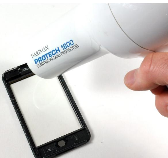
*(i)* The front panel is held in place by a heat-sensitive glue that bonds the panel to the frame on all four sides.
