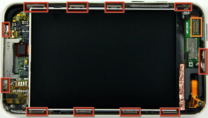
**i** The glass front panel on the second generation Touch has a plastic frame glued both to its outer edge and also under the wide black strips at the top and bottom of the device. The frame also has a rubber strip that surrounds the edge of the glass panel.
