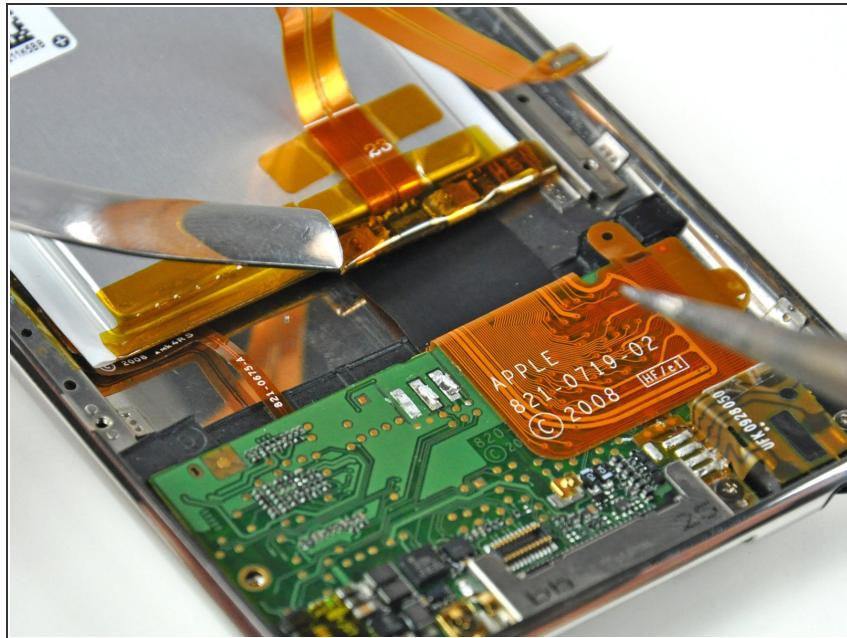
ⓘ At this point, the battery should be free from the logic board.
