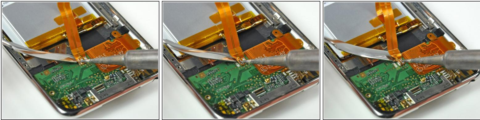
① The battery on the third generation Touch is attached via solder pads with small holes that go *through* the battery ribbon cable and attach to flat pads on the face of the logic board. In this step, you will heat each solder pad individually while using a metal spudger to pry it up from the logic board.
