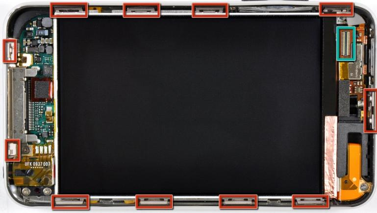
**i** The glass front panel on the third generation Touch has a plastic frame glued both to its outer edge and also under the wide black strips at the top and bottom of the device.
