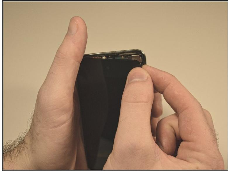
**⚠** Use extreme caution when handling the front panel assembly, as it is attached to the rest of the Touch by the very delicate digitizer cable.
