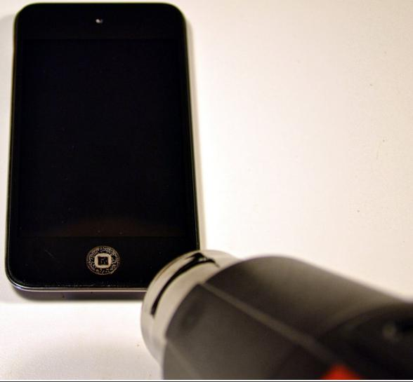
**i** The iPod Touch 4th Generation front panel is attached to the rear case by an adhesive. The use of a heat gun to soften the adhesive is highly recommended.
