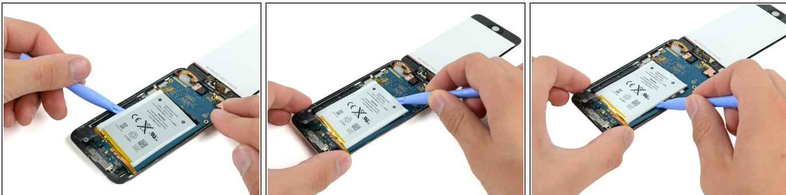
⚠ In the next few steps, you will loosen the adhesive from underneath the battery, the logic board, and the frame under the battery. Do this slowly, carefully, and evenly. Take care not to puncture the battery or bend the logic board.
