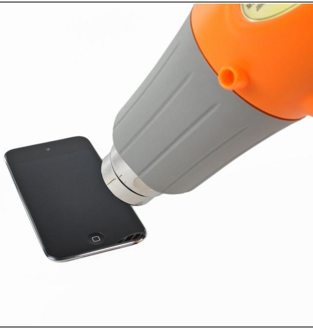
**i** The iPod Touch 4th Generation front panel is attached to the rear case by adhesive. The use of a heat gun to soften the adhesive is highly recommended.
