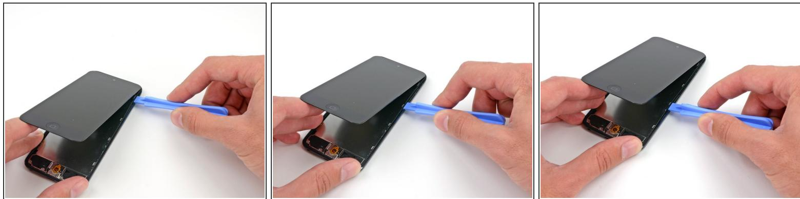
*(i)* In the following steps, you will be loosening and freeing the plastic frame that surrounds the screen. It is connected to the rear case with several clips.
