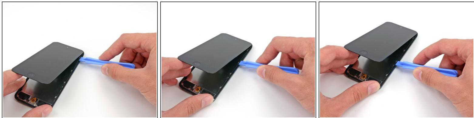
ⓘ In the following steps, you will be loosening and freeing the plastic frame that surrounds the screen. It is connected to the rear case with several clips.
