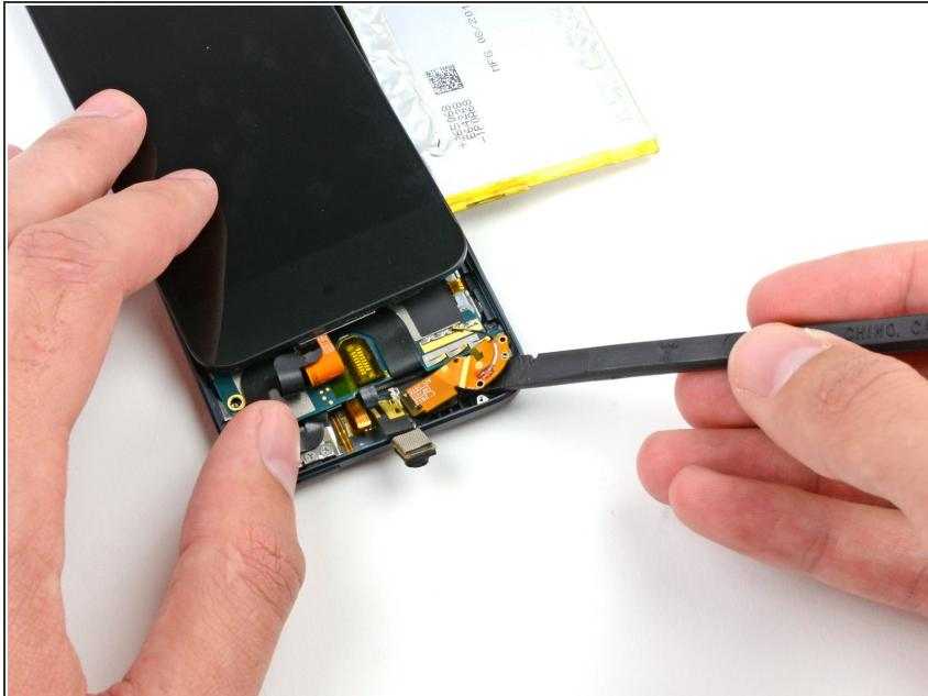
*(i)* Flip the screen back over onto the rest of the iPod to expose the edge of the antenna.
