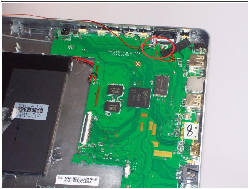
**⚠** Locate the two speakers and using the soldering iron and solder sucker carefully remove the solder that binds the two speakers down.
