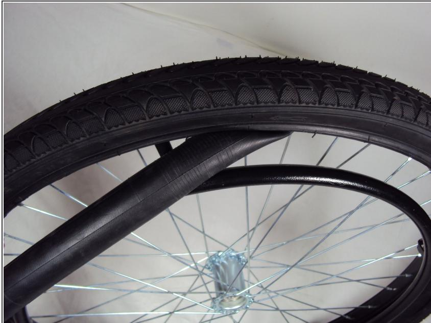
*(i)* Before replacing the tube, feel along the tire to check for and remove any objects stuck in the tire.
