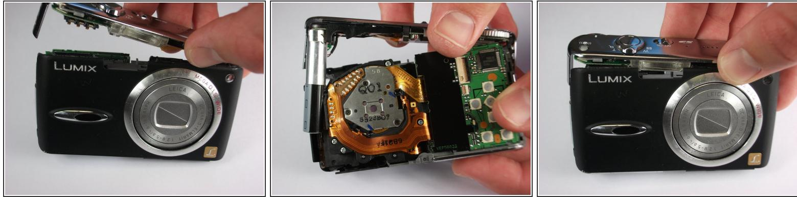
⚠ Carefully remove the upper assembly, which houses the buttons and the flash battery.
