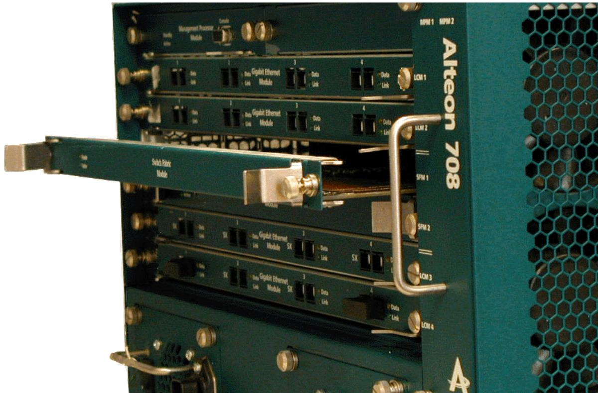
**Figure 25** Inserting the Switch Fabric Module
