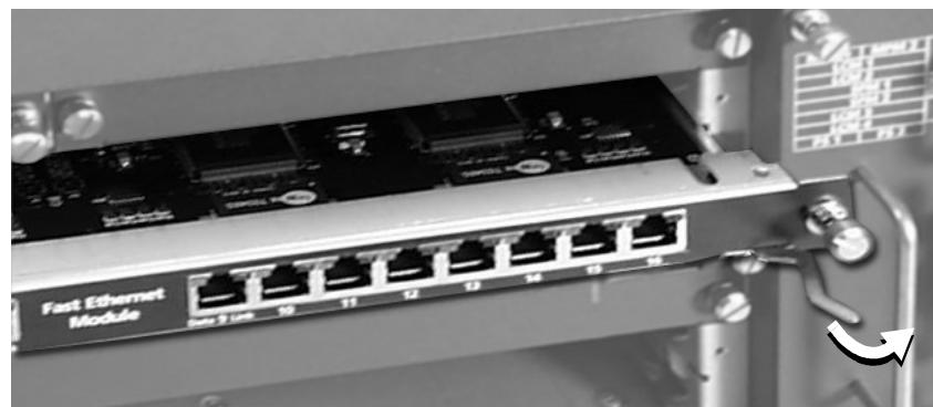
**Figure 14** Open the Insertion Levers
