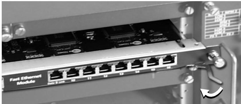
**Figure 15** Close the Insertion Levers to Mate the Module
