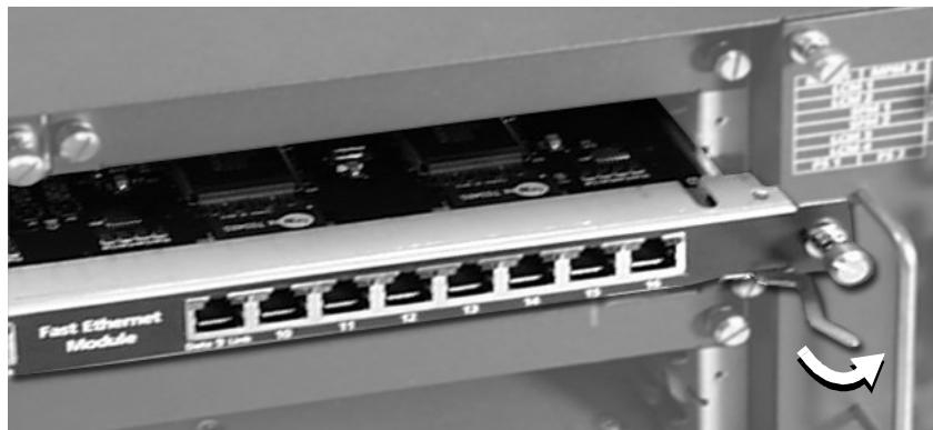
**Figure 16** Use the Ejection Levers to Free the Line-Card Module
