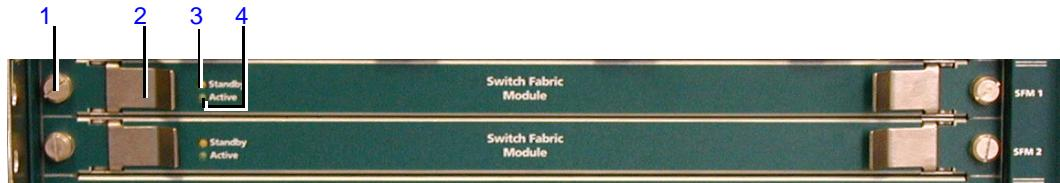
**Figure 24** Switch Fabric Module Faceplates
