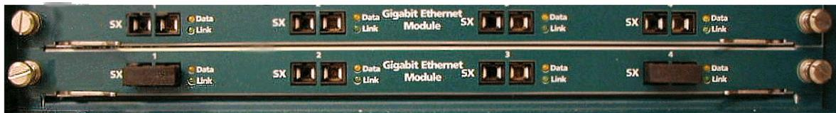
**Figure 20** 1000Base-SX Gigabit Ethernet Fiber Optic Line-Card Module Faceplate
