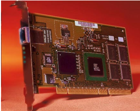
Figure 1 The ACEnic 10/100/1000Base-T Gigabit Ethernet Adapter
